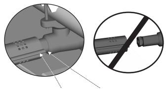
Correctly assembled burner tube and valve.
